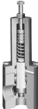
Prevent over pressures, maintain back pressures or automatic by-pass in vessels and piping. Series RVDM (not shown) in-line pattern has a frictionless rolling diaphragm design for sensitive operation. Series RVT is an angle-pattern design. Settings from 5 to 100 PSI. Fail Dry®, 1/2" to 2". Series RVD angle pattern diaphragm design (not shown) 1/8" to 1/2" NPT, 50 to 150 PSI. Series RVTX offered in 3" NPT.
