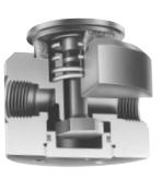
Normally-closed MFR palm or foot operated valves are the answer for applications where hand or hands must be kept free for other functions. Automatic spring-return closes valve bubble-tight seal. Low-friction design; no wetted metals. 1/2" and 3/4" sizes. Cv 2.5 and 5.0; 150 PSI max; vacuum service available.
