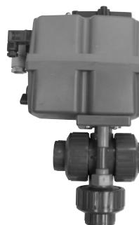
Simple attachment to the valve body mounting lugs. Available with fail-safe and 4-20 mA or 0-10 VDC digital control options. Two actuator sizes for the valve range of 1/2" through 4".
