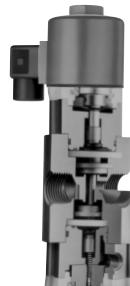
Normally-open, direct-acting Series EASY-NO closes when energized. Designed for applications that must have continued flow in the event of a power failure. Suitable for pressure, drain or vacuum service with pressures to 70 PSI. Direct-acting Series THP is a multi-purpose valve suitable for inlet and backpressures to 100 PSI; it can function as a three-way, normally-open, or normally-closed valve. Both EASY-NO and THP are available in 1/4" and 1/2" sizes in PVC.
