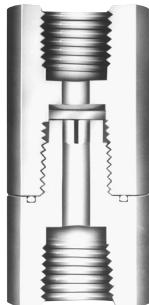
Series CK is a machined PTFE valve that features the same normally-closed diaphragm design as Series CKM, available in 3/4" and 1" sizes. Series CKD is a normally-open diaphragm check valve that is ideal for ultra-low pressure or flow, requires .5 PSI to close. Sizes 1/4" and 1/2" in PVC, Natural Polypro, PTFE and PVDF.
