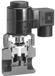
This compact, direct-acting design provides a cost effective solution for high pressure rated applications, where space is limited. Patented Fail-Dry® safety design. For virtually all type solutions: acids, caustics, solvents, chlorine solutions and ultra-pure liquids. 2,000,000 cycle life. Sizes 1/4" and 1/2". Cv of 0.5 with 3/16" orifice; 0.8 with 1/4" orifice. PVC, CPVC, Natural Polypro, PVDF.
