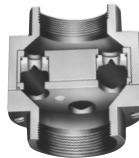
Automatic, tamper-proof valves maintain a constant flow regardless of inlet pressure changes between 15 and 100 PSI. No metal in contact with liquid. Maintains pre-determined flow rates from 1/4 to 120 GPM. Sizes 1/4" to 3".
