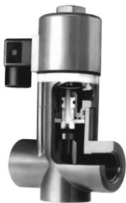
Direct-acting valve for severe service applications with virtually all solutions (acids, caustic, etc.). Unique "Bellows" design provides dynamic barrier seal, prevents leaking of emissions. 2,000,000 cycle life. Fail-Dry® safety design. Sizes 1/4" to 1". Cv from 1.1 to 4.7, orifice from 3/8" to 11/16". PVC, CPVC, Glass-filled Polypro, PVDF.
