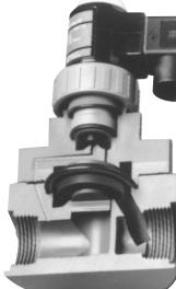
High pressure, high flow capability. Pilot-operated design requires 5 PSI differential across the valve. Rated for inlet pressures 5 to 140 PSI, back-pressures to 70 PSI. Cv's from 5.2 to 80. Patented Fail-Dry® safety design. PTFE bellows barrier type seal. For all type solutions. Sizes 1/2" to 3". PVC, CPVC, Natural Polypro, PVDF.
