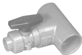
Revolutionary ball valve adapter eliminates weakness inherent to lateral drops; installs easily into the tee without additional fittings. Also an ideal replacement for costly zero dead-leg valves. 1/2" to 2" Ball Valves sizes. 3/4" to 3" tee adapters standard; other sizes consult factory. Available in PVC, CPVC, PVDF and natural polypropylene, socket or butt fusion.
