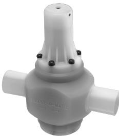
The ultimate high purity pressure regulators. PRH-U features machined Kynar 740 body with metal ion-free EPDM elastomer and non-rising adjustment. UPR has convoluted TFM diaphragm and no external fasteners and is designed to meet SEMI F-57 specifications. PRH-U regulator setting from 10 to 125 PSI, sizes 1/4" to 3". UPR setting from 5 to 100 PSI, sizes 1/4" to 2". Both PRH-U and UPR include choice of spigot types. Also include
