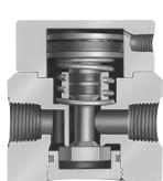
BSR air-operated valves are normally-closed, ideal for purity and corrosive applications. Features low friction design bubble-tight seal, no wetted metals. 1/2" and 3/4" sizes. Cv 2.5 and 5.0; 150 PSI max; vacuum service available.
