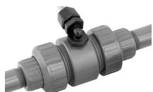
Air-operated valves "pinch" sleeve to shut off flow; ideal when slurries or particulate might prevent bubble-tight closure in a regular seat and seal design. HSA is an inline design that closes a Patent Pending articulated sleeve molded of EPDMh2, 1/2" to 1" connections of PVC, CPVC, natural polypro or PVDF. HTA pinches user supplied tubing from 3/8" to 1/2" diameter.
