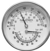
All-in-one pressure and temperature gauge with extra low-profile probe. Suitable for applications that can withstand wetted metal. Steel case and stainless steel connection; multiple pressure ranges available in 2 1/2" or 3" gauge face.
