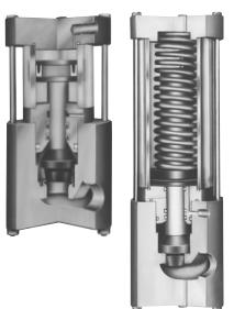
2-way globe-type shutoff valves feature PTFE shaft design, Fail Dry® design and clear acrylic air cylinder shows valve position, all standard. Ultra heavy-duty valves with decades of proven rugged performance. Series BAT is double-acting air to open, air to close. Series BLT uses the liquid process pressure to open, air to close. Series BST is air x spring, normally closed or normally open. Sizes 1/2" through 2".
