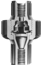
Leak-proof check valves prevent reverse flow of water, extremely corrosive and ultra-pure liquids. Self-sealing designs allow mounting in any position. Unique molded diaphragm in sizes 1/2", 3/4" and 1"; self-guided poppet in 1 1/2", 2" and 3". Both styles are normally-closed – no reverse pressure required. They operate silently, and seat in the same location every time. PVC, CPVC, Polypro, PVDF.
