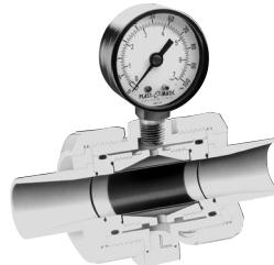
Unique in-line design eliminates "dead leg" that can harbor bacterial growth and contamination. Unpigmented thermoplastic material; FKM or metal ion-free EPDM. Special flexible elastomer spool separates system liquid from gauge fill liquid and assures accurate reading. Adaptable to existing piping systems. Sizes: 1/2" to 2".
